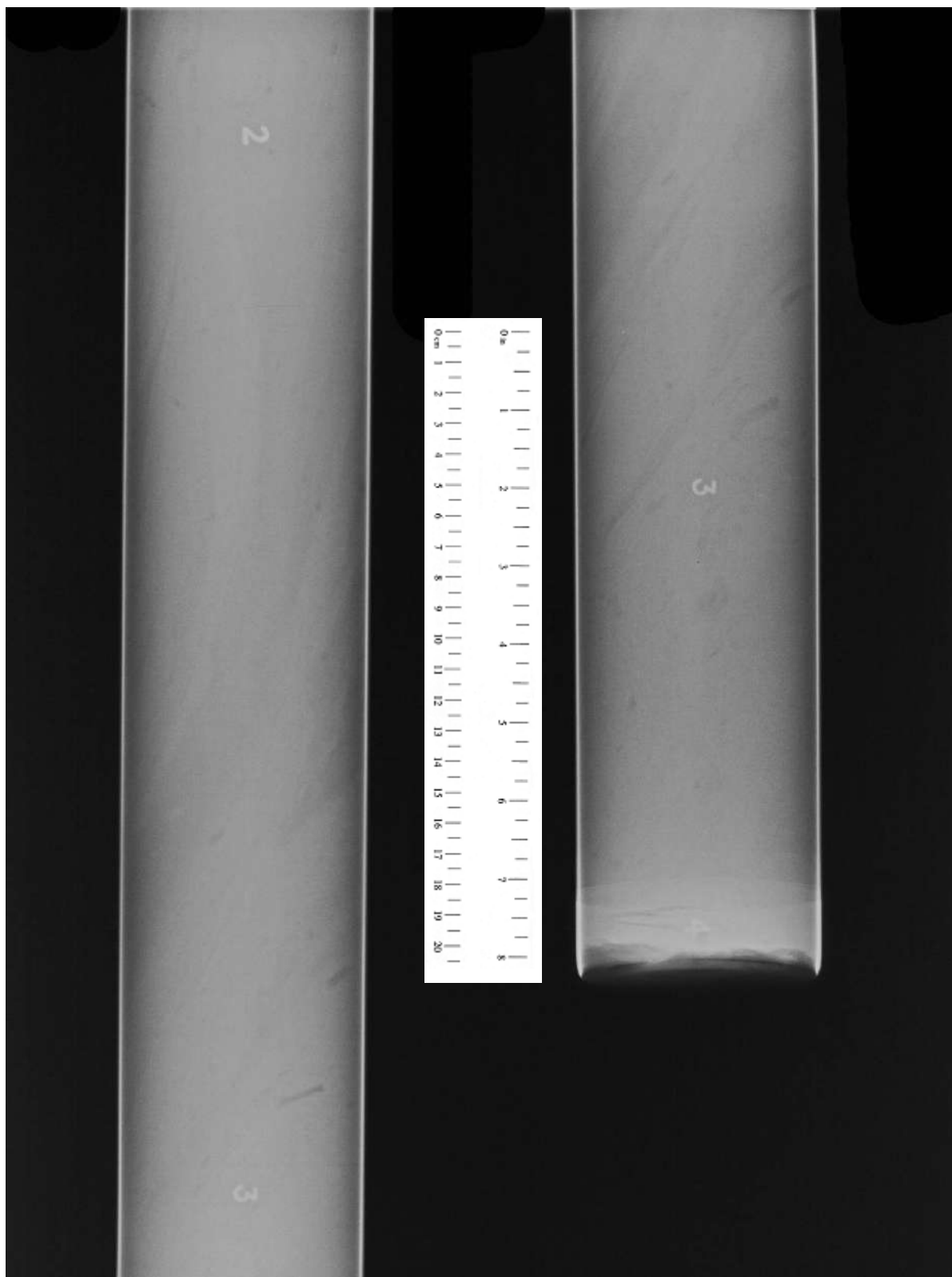
X-RAY RADIOGRAPHY IMAGES BORING B-191, SAMPLE S-36, DEPTH 112.2 – 114.2 FT ONSHORE LNG FACILITIES ALASKA LNG PROJECT NIKISKI, ALASKA
