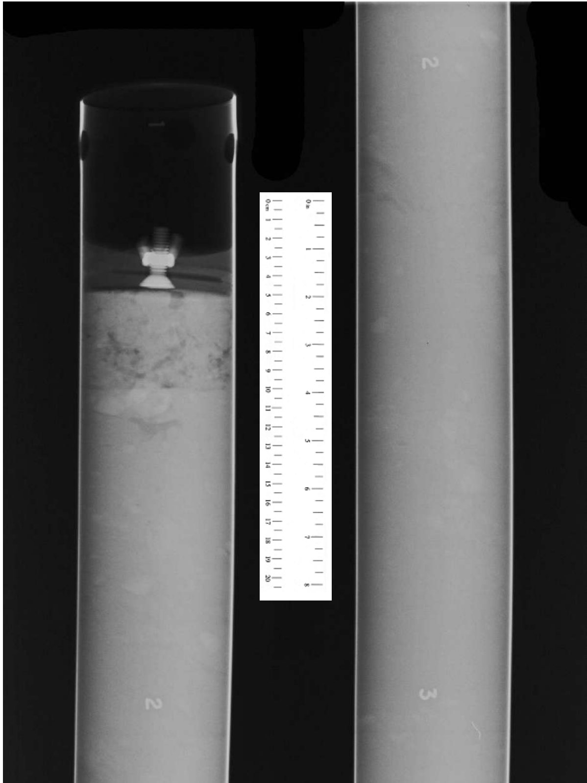
X-RAY RADIOGRAPHY IMAGES BORING B-191, SAMPLE S-15, DEPTH 46.0 – 48.0 FT ONSHORE LNG FACILITIES ALASKA LNG PROJECT NIKISKI, ALASKA
