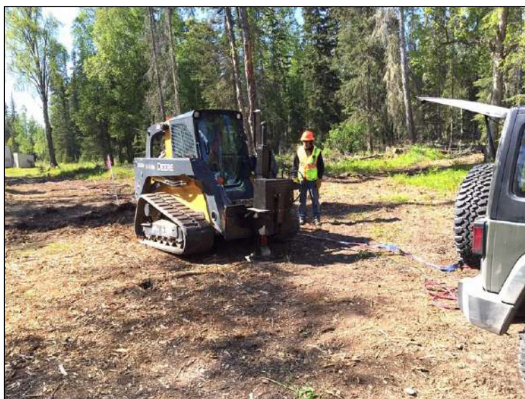
A 200-lb accelerated weight drop (AWD) mounted on skid steer, sourcing on Line EW-3.
