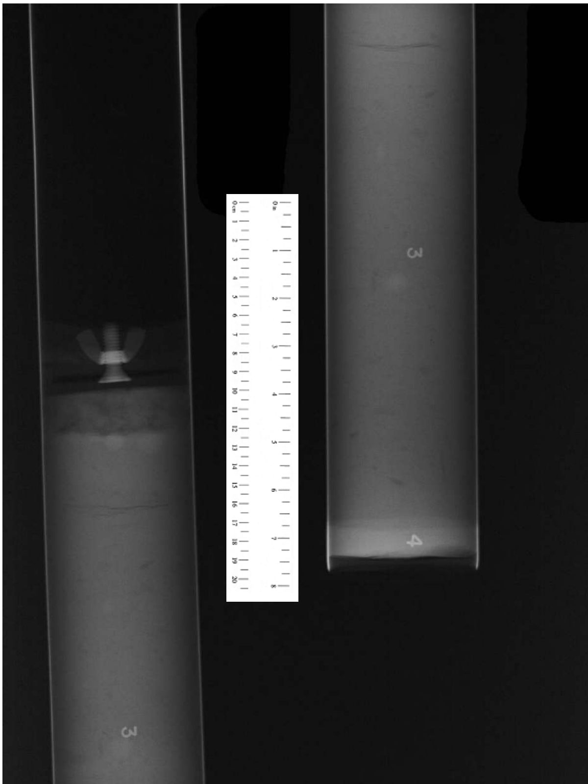
X-RAY RADIOGRAPHY IMAGES BORING B-197, SAMPLE S-49, DEPTH 229.0 – 230.0 FT ONSHORE LNG FACILITIES ALASKA LNG PROJECT NIKISKI, ALASKA
