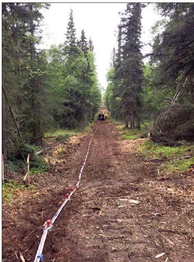
Land streamer consisting of 72 geophones spaced at 1 meter intervals along a Teflon-coated strap, is towed behind a vehicle to advance the array.
