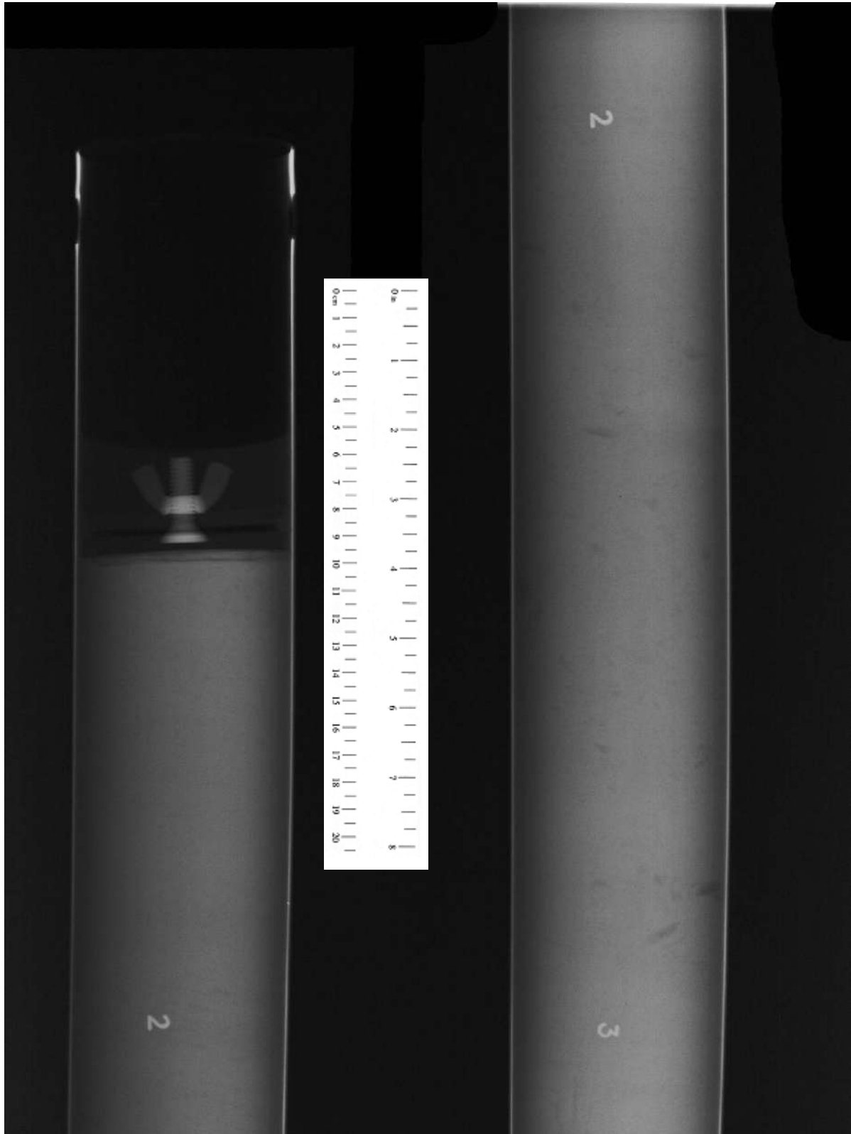
X-RAY RADIOGRAPHY IMAGES BORING B-192, SAMPLE S-45, DEPTH 219.0 – 220.9 FT ONSHORE LNG FACILITIES ALASKA LNG PROJECT NIKISKI, ALASKA
