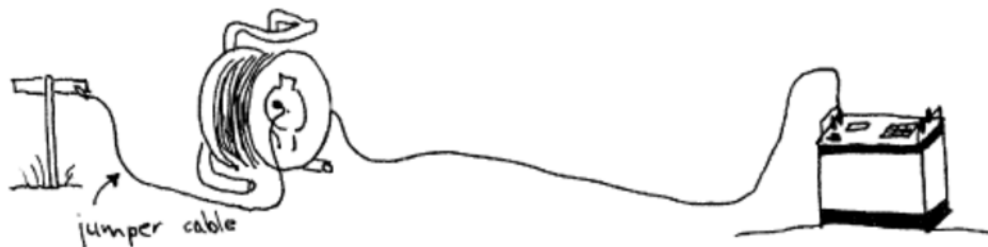
Schematic showing connection of sounding cables, jumper and instrument
