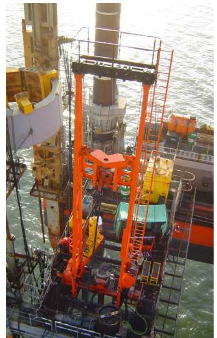
CR2 Marine Drill at Barrow OWF
