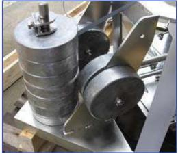
The Day Grab has 2 identical weight stations, each side is capable of holding 7 pcs weights and an additional mounting of vertical weights. (2 x 4 pcs).
