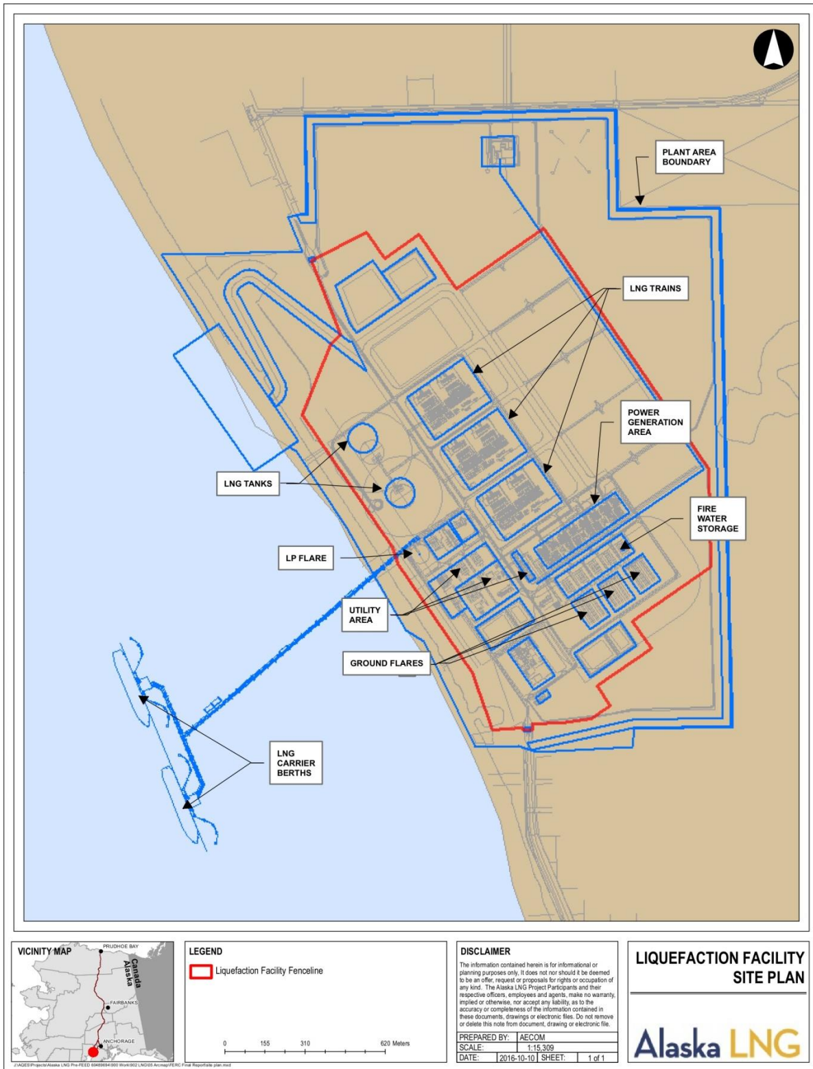
Figure 1-2: Project Proposed Liquefaction Facility Site Plan
