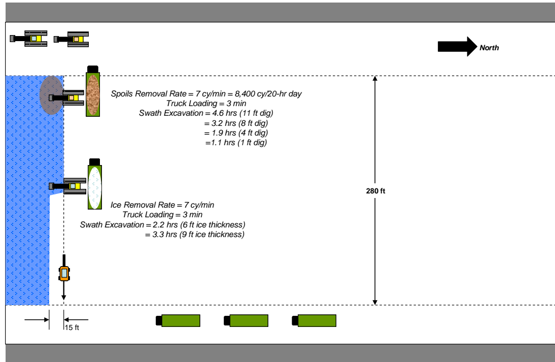
Figure 5-3. Remove Sea Ice and Dredge Seabed
