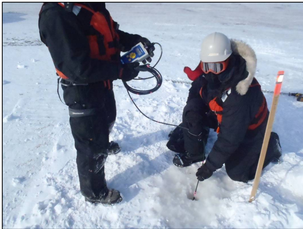
Figure 4-20. Deployment of Turbidity Sensor through Hole Augured in Sea Ice
