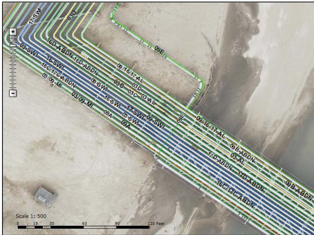
Figure 19: Sagavanirktok River Pipe Bridge Existing Pipeline Identification
