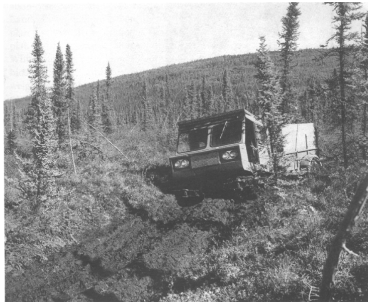
Off-Road Vehicle trail in permafrost during summer of 1977, after two seasons' traffic
